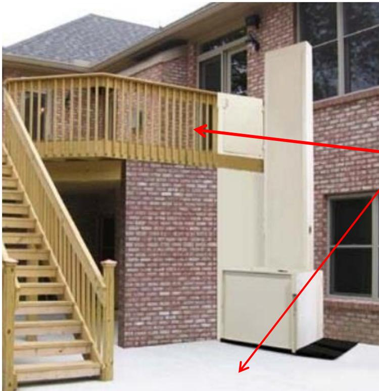
Be sure there is an accessible route to the lift and that there is enough room for someone in a wheelchair to access the lift from the top and bottom!
